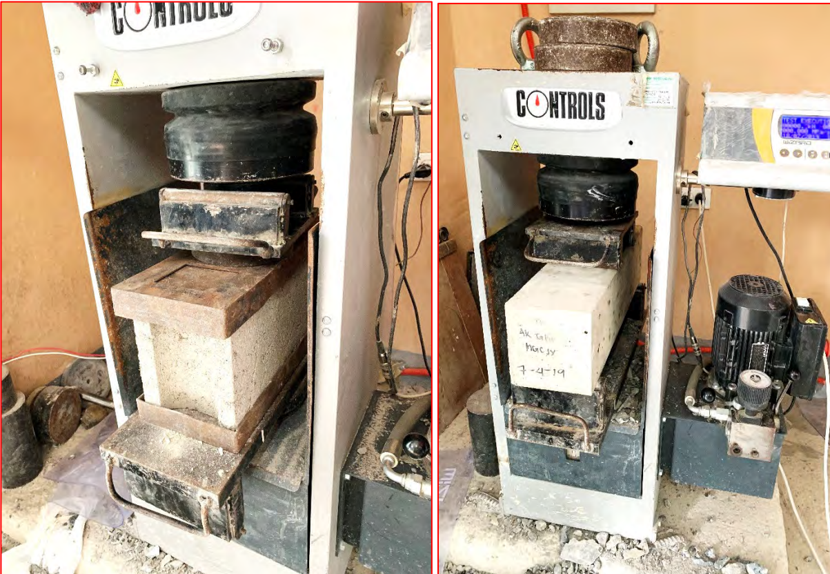
Figure 26: Concrete Masonry Unit(CMU) and Beam Sample testing.
